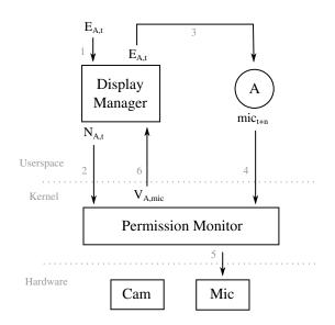
Figure 1. Dynamic access control over privacy-sensitive hardware devices.
