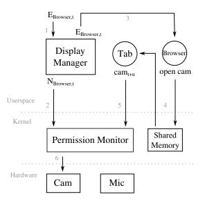
Figure 4. A multi-process browser, components of which communicate via shared memory IPC. This example illustrates the need for interposing on IPC endpoints to propagate interaction information.
