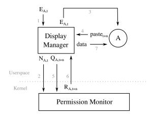
Figure 2. Protecting copy & paste operations against clipboard sniffing.
