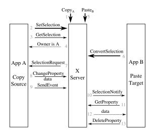
Figure 6. Protocol diagram for the X11 copy & paste operation. Modified steps are highlighted in bold.
